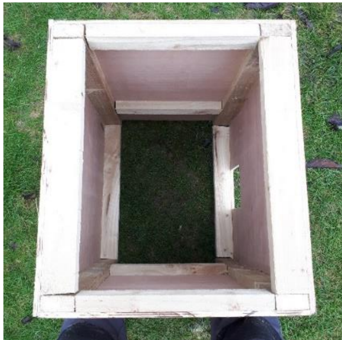
View of the bottom of the box (box is upside-down) before floor has been attached (Image: Alan McCarthy)
