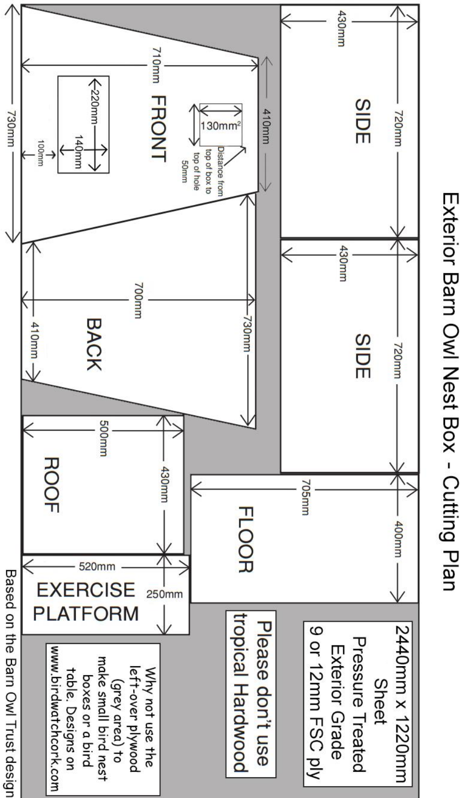
Figure 5. Cutting plan for exterior barn owl nest box
